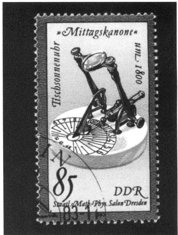
Fig.2 Noon gun and horizontal sundial of 1800 on an East German stamp of 1983. Note the latitude of 51° 13' 48"
